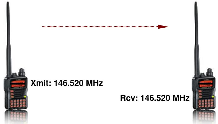
Simplex – both radios are transmitting and receiving on the same frequency.
