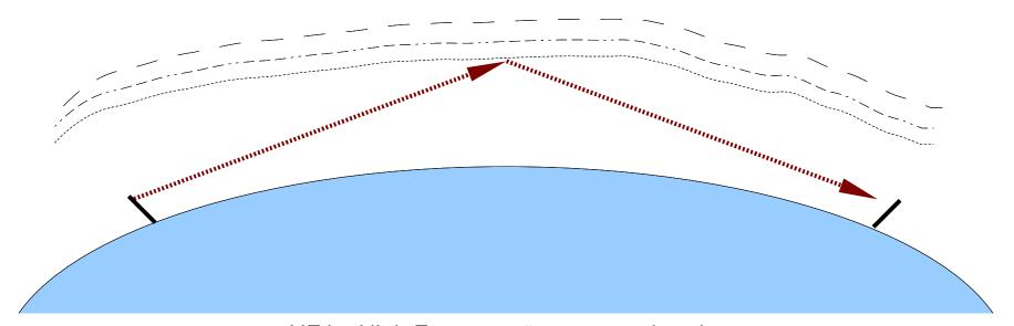
HF is "High Frequency" – amateur bands: 160 meters (1.8MHz – 2.0MHz) 80/75 meters (3.5MHz – 4.0MHz) 60 meters (5.3MHz – 5.4Mhz) 40 meters (7.0MHz – 7.3MHz) 30 meters (10.10MHz – 10.15MHz) 20 meters (14.00MHz – 14.35MHz) 17 meters (18.068MHz – 18.168MHz) 15 meters (21.00MHz – 21.45MHz) 12 meters (24.89MHz – 29.99MHz) 10 meters (28.0MHz - 29.7MHz)
