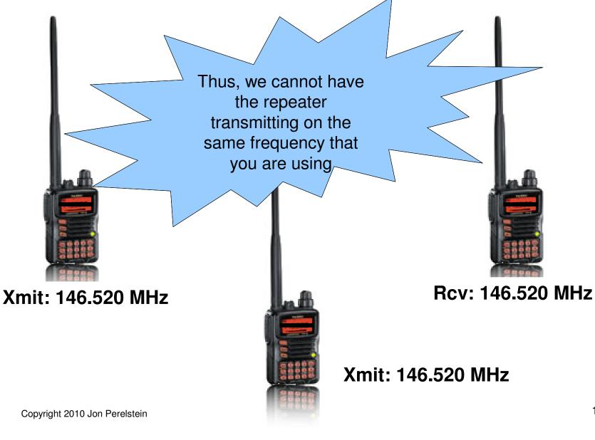
The sender (you) and the repeater each have to transmit on a different frequency
